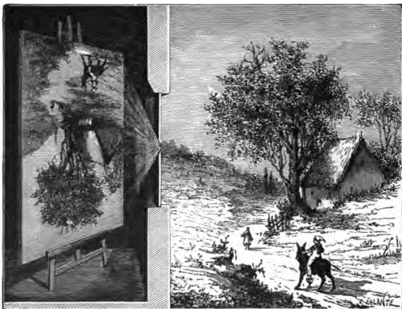
FIG. 75. A PICTURE OF THE LANDSCAPE FORMED INSIDE A DARK ROOM ( Camera obscura ) BY LIGHT THAT PASSES THROUGH A VERY SMALL HOLE
